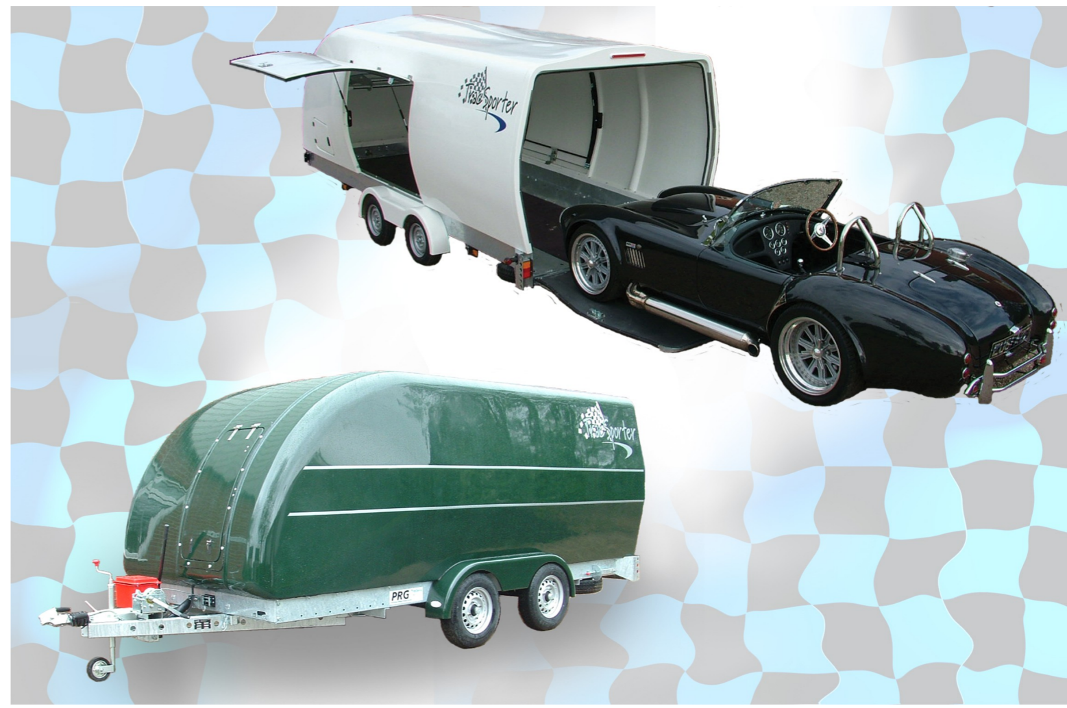
Hydraulic tilt bed operation with dual action hand pump, allowing the shallowest loading angles on the market. We also have an electric tilt bed option.
